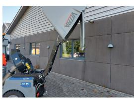
The collector has unloading height of up to 190 cm, to ensure a lot of tipping possibilities for the driver.
